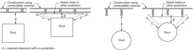
B = reduced clearance with no protection B = reduced clearance permitted
